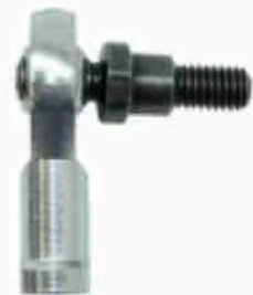
· Type rod end: inner thread · Length: 27 mm · Thread: M5/M6 · RH/LH thread: RH Used on HR21 REF 150TA9836
